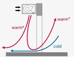
The air speed is too high. The airflow splits when it hits the floor. Warm air enters the cooled or unheated room. The air speed must be reduced.
