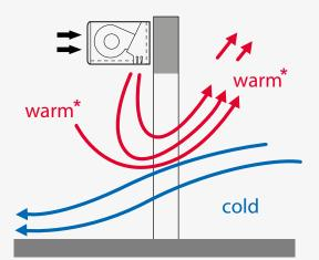
The air speed is too low. The airflow does not reach the floor. Cold air can escape below the airflow. The air speed must be increased.
