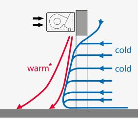
The air speed and the discharge angle are ideal. The airflow is located in front of the door opening. The cold air cannot escape. Warm air cannot penetrate the cold or unheated room.
